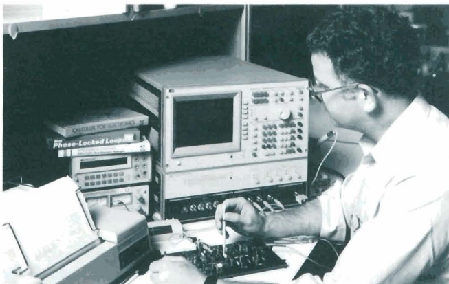
The HP 4194A Impedance/Gain-Phase Analyzer tests materials, components, ICs and circuits to 40 MHz for impedance measurements and 100 MHz for gain-phase measurements.
