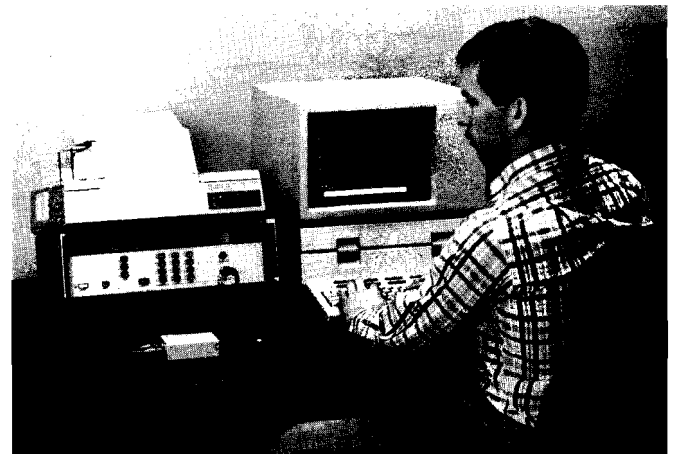
VCO characterization and measurement to 40 GHz are simplified with the HP 5352A Microwave Frequency Counter
